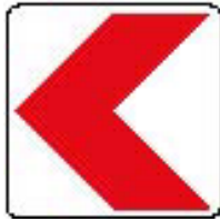
Sharp Curve Chevron Sign
