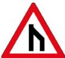
End of Dual Roadway Sign
